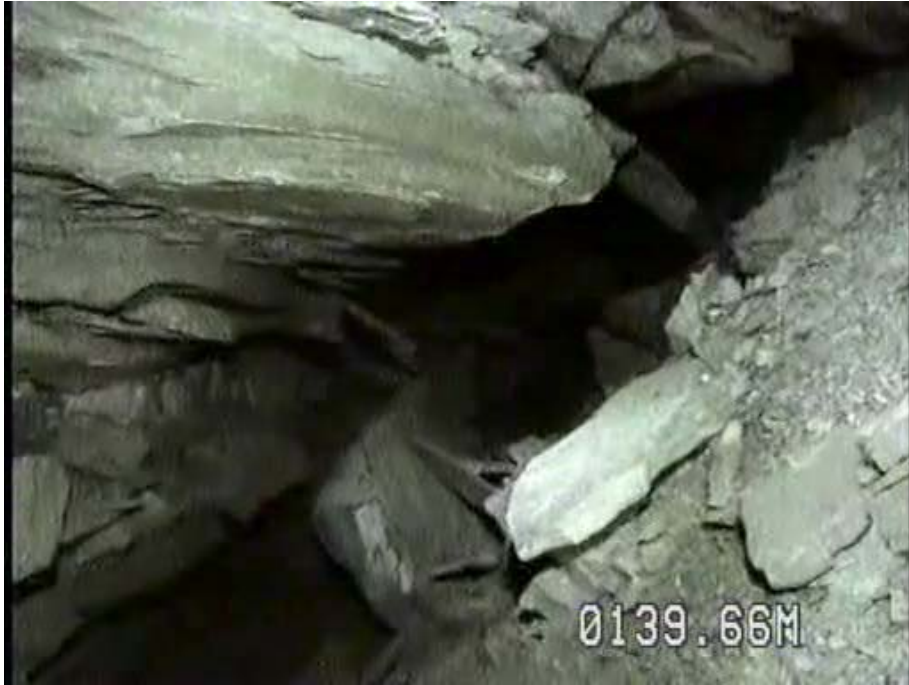
Figure 4.15. Degas Hole 11 Obstructed by rock fall at 139 Meters
